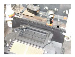
28. Apply 1/2" gasket along this entire edge. Use two pieces of masking tape to hold the gasket in place. The masking tape will burn off during normal stove use.
