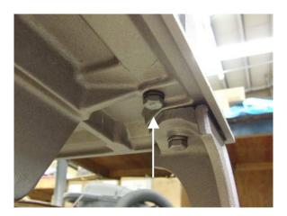
11. From the top of the stove locate the lift guide that connects to the bypass cover. It is the cast iron loop that is fastened to the bypass cover with two bolts. The bypass cover is the "bull horn shaped" door that opens to allow gas to bypass the catalytic combustor. Remove the two bolts with a 1/2" wrench or socket and then push the lift guide back out of the way toward the rear of the stove.
