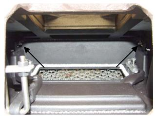
5. Lift the top off the stove. This piece is heavy. Lift it straight up and then place it aside.
