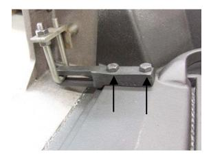
12. At the top of the stove, remove the four hex head bolts that hold the combustor pan in place. These are located at each of the outside corners of the combustor pan.
