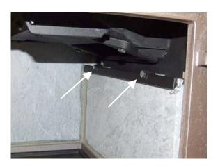
38. Use the shank of a 1/4" drill bit as a measuring device to reset the space between the front edge of the air guide and the glass panel. The spacing should be adjusted so that the drill bit may move between the two with just a slight bit of friction. Tighten the two air chute bolts securely with the proper 1/4" spacing.
