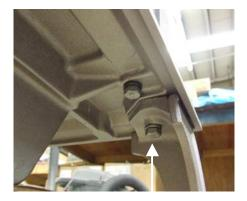
37. Reinstall the rear stone retainer. Place the bolts through the retainer and into the extended rear wall of the combustor pan. Tighten the bolts incrementally and evenly.
