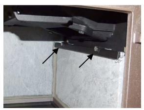
8. While inside the firebox locate the 2 bolts on the backside of the doorframe. Loosen the locking nuts clockwise, then turn the mounting bolts counterclockwise, using a 1/2" wrench, to release them from the combustor pan.
