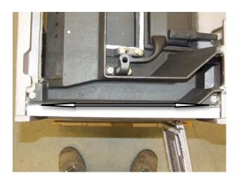
42. Remove all of the old glue and gasket material from the underside of the top assembly using a flat blade screwdriver or small Dremel like tool.
