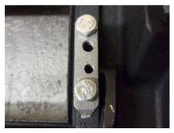
22. Once the retainers are fastened securely start the "adjustment" screws in the center of each retainer, but only by a thread or two. Now lift the bypass cover from the bottom side upward so that the two pivot points or "bull horns" are pressed up against the bottom side of the retainers. With the cover held in this position, tighten the
