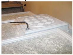
2. Remove the stainless steel combustor shield that is attached to the catalytic combustor assembly using a 7/16" nut driver or short wrench.
