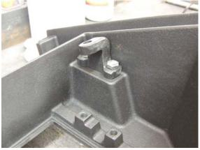
15.Transfer the air chute from the original pan to the new one, but <u>do not tighten the bolts completely</u> as the chute will have to be adjusted after the pan is installed. The air chute is the long cast iron plate that protrudes from the front edge of the combustor pan and is fastened with two bolts and two flat washers that come up through the bottom side of the chute and into the bottom side of the front edge of the combustor pan.
