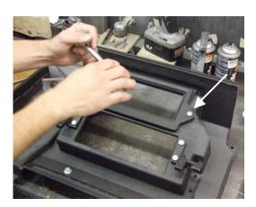
19. Remove the two scoop supports (1/2" socket or wrench) from the original pan noting the position of each. Install the supports on the new pan, pushing each of them outward as they are installed, so that there is as much distance between them as possible for proper fit of the combustor scoop. Place the scoop on the supports to test
