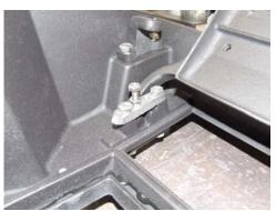
23. Apply gasket glue along the channel around the combustor assembly port and insert 1/4" gasket along the channel, with the split in the gasket at any of the four corners.
